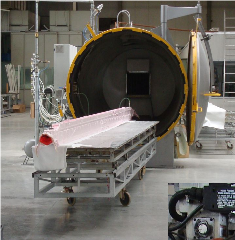
After lamination in White Room, the mast is fully post-cured in autoclave
